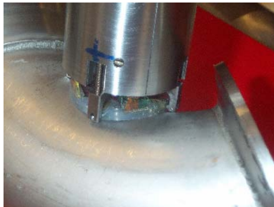
Figure 8. Smart phased array transducer located on the intrados of an elbow with 70mm diameter and 60mm of bending radius.
